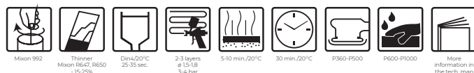
Mixon 992 Thinner Mixon R647, R650 -15-25% Diluent 20°C 25-35 sec. 2-3 layers ø 1.5-1.8 3-4 bar 5-10 min./20°C 30 min./20°C P360-P500 P600-P1000 More information in the tech. map
