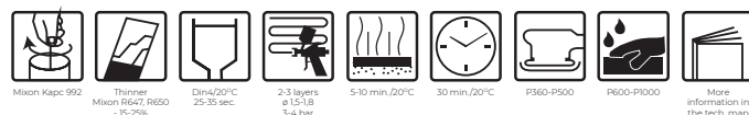
Mixon Kapc 992 Thinner Mixon R647, R650 -15-25% Diluent 20°C 25-35 sec. 2-3 layers ø 1.5-1.8 3-4 bar 5-10 min./20°C 30 min./20°C P360-P500 P600-P1000 More information in the tech. map
